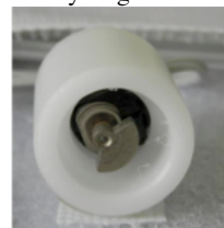
Figure 3 – Eccentric Rotating Mass Based Tactor
